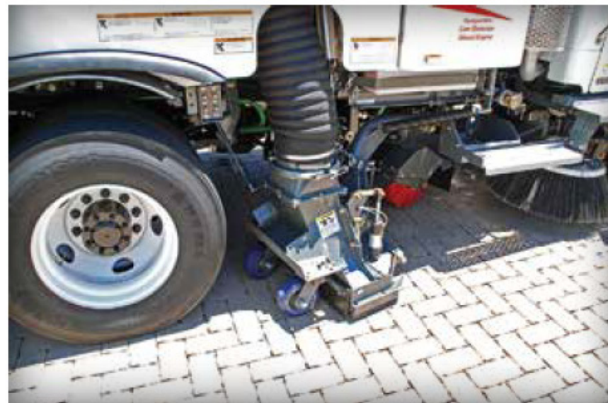
Figure 22. A true vacuum machine cleaning neglected PICP.
