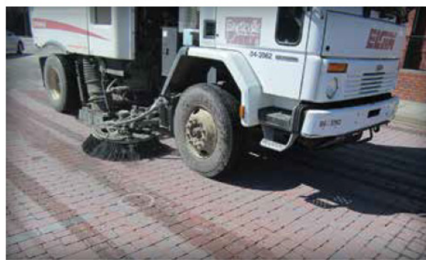
8.2 Figure 21. A regenerative air machine cleaning a PICP parking lot.
