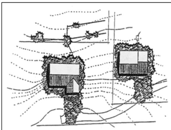
**Figure 2.14 Establishing Limits of Clearing**
