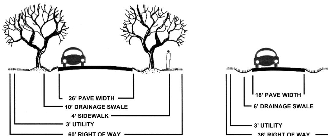
**Figure 2.19 Potential Design Options for Narrower Roadway Widths**
