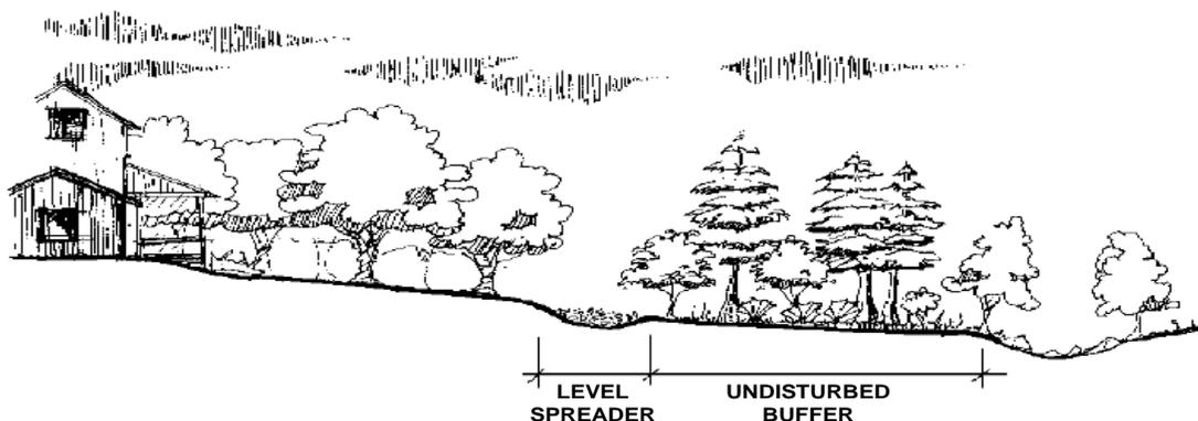
**Figure 2.29 Use of a Level Spreader with a Riparian Buffer**
