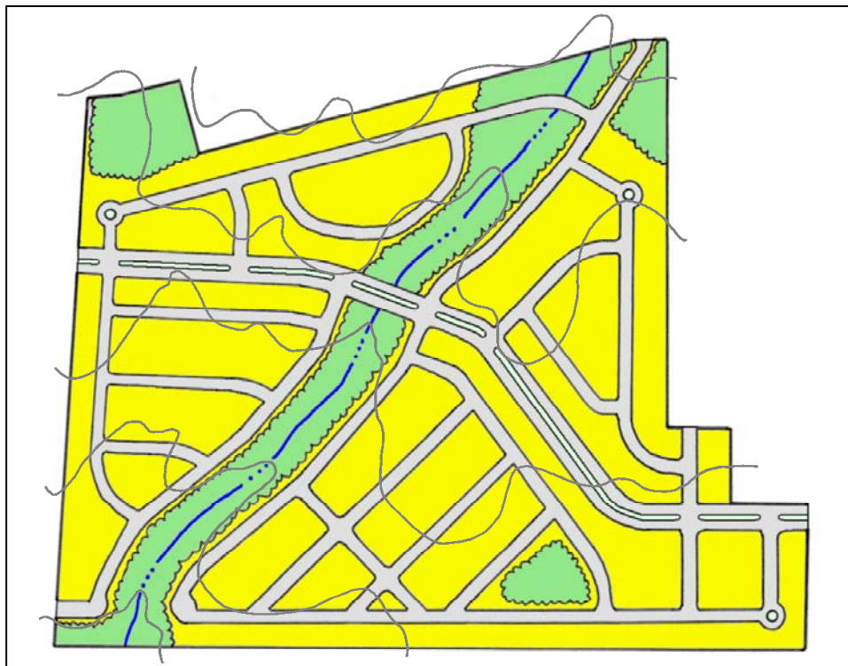
Figure 1.3.2-11 A Subdivision Design for Flat Terrain Uses a Fluid Grid Layout that is Interrupted by the Stream Corridor
