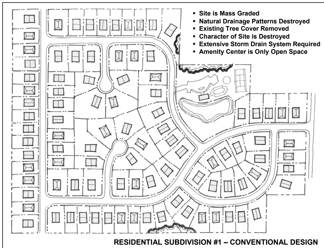
Figure 1.3.3-1 Comparison of a Traditional Residential Subdivision Design (above) with an Innovative Site Plan Developed Using integrated Site Design Practices (below).
